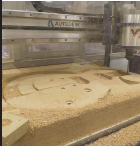
The wood is being processed through a CNC milling machine.
