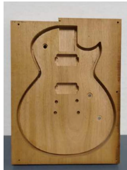
After the milling operation, front side.
