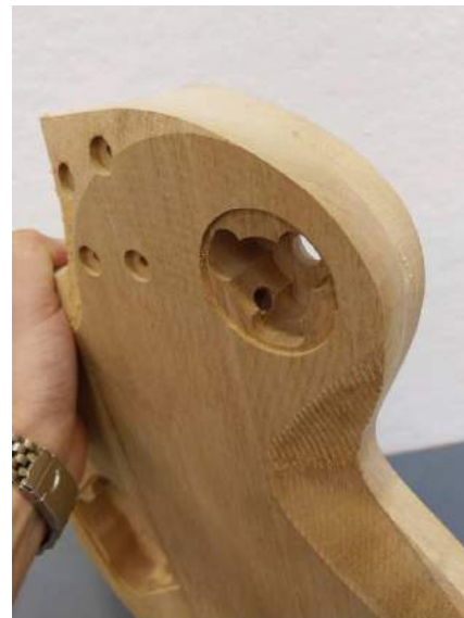
After the milling operation, back side.
