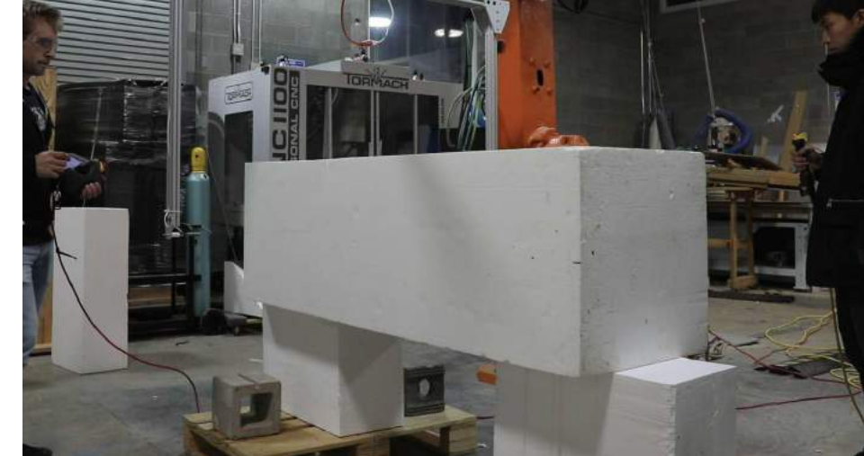
First cut operation, to form the seat and to cut down the block of foam to size.
